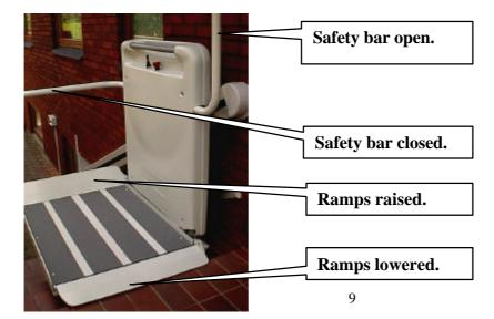
• NB. Never leave the platform until the ramps have been fully lowered and are firmly supported by the stairs.
