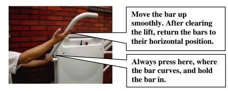
• The platform can be released manually by raising it to its vertical position to allow free passage on the stairs.
