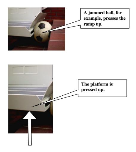
• The safety bars stop automatically if they are prevented from moving freely. Restart the bars by activating the joystick.
