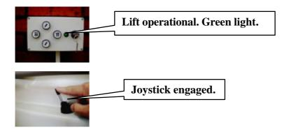
• The safety bars and ramps close automatically when the joystick is engaged. The lift will not run until the safety bars and ramps are in closed position.
