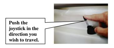
G. The safety bars close and the ramps are raised automatically. The lift then starts and continues to run until it reaches the other end of the stairs or for as long as the joystick is engaged.
